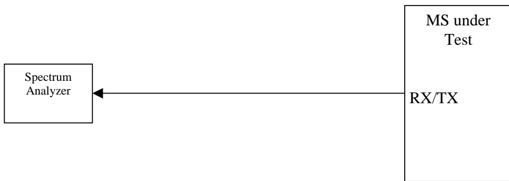
Figure A.8: Connection for Spurious Emission Test
