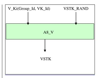
The GCR sends the parameters Group Id, VK Id, VSTK RAND, VSTK, A5 Id via the anchor-MSC and the relay-MSC's to the BSS. The BSS signals the Group Id, VSTK RAND and VK Id to the ME.
