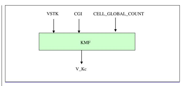
To provide the required information to the ME the parameters CELL GLOBAL COUNT and CGI are included in various messages from the BSS to the ME (I.e. CELL GLOBAL COUNT on the NCH, FACCH and PCH, and the CGI on the BCCH and the FACCH).
