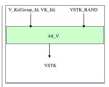
The GCR sends the parameters Group Id, VK Id, VSTK RAND, VSTK, A5 Id via the anchor-MSC and the relay-MSC's to the BSS. The BSS signals the Group Id, VSTK RAND and VK Id to the ME.
