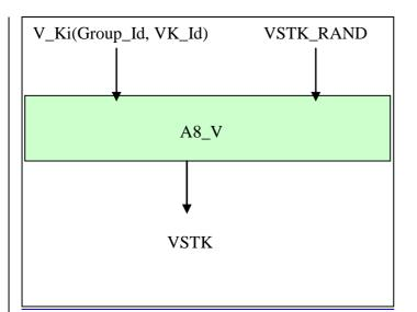
The GCR sends the parameters Group Id, VK Id, VSTK RAND, VSTK, A5 Id via the anchor-MSC and the relay-MSC's to the BSS. The BSS signals the Group Id, VSTK RAND and VK Id to the ME.
