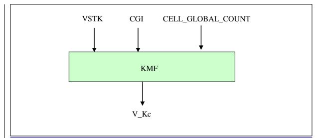
To provide the required information to the ME the parameters CELL GLOBAL COUNT and CGI are included in various messages from the BSS to the ME (I.e. on the NCH, FACCH and PCH).
