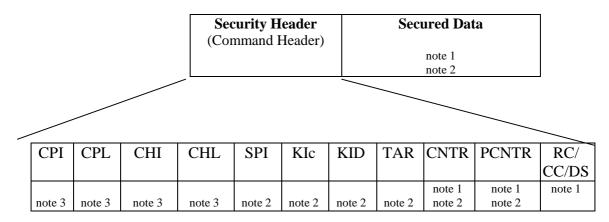
NOTE 1: These fields are included in the data to be ciphered if ciphering is indicated in the Security Header.
