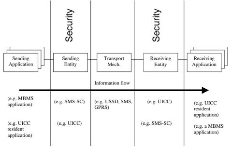
The Sending Entity and the Receiving Entity establish a secure communication by exchanging Secured Packets according to TS 102 225.
