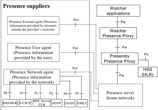
Interfaces Ph, Pi, Pc, Pg, Pk and Pl are based on existing R5 procedures e.g. CAMEL, MAP, CAP, RADIUS, ISC, Cx, Sh.
