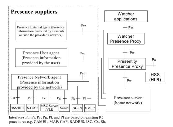
Figure 1: Reference architecture to support a presence service [TS23141]
