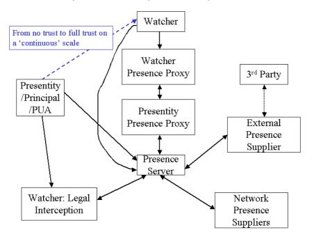
It is assumed that a 3<sup>rd</sup> party is not necessarily situated in a 3G network and therefore no trust establishment has been stated here. Presumably any operator setting up a relationship with a 3<sup>rd</sup> party needs to ensure that necessary considerations around trust and security measures are considered.
