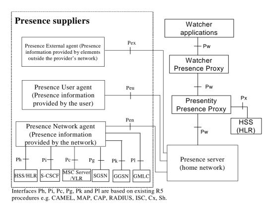
Figure 1: Reference architecture to support a presence service [TS23141]
