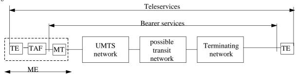
ME: Mobile StationMT: Mobile TerminationTE: Terminal EquipmentTAF: Teminal Adaption Function
