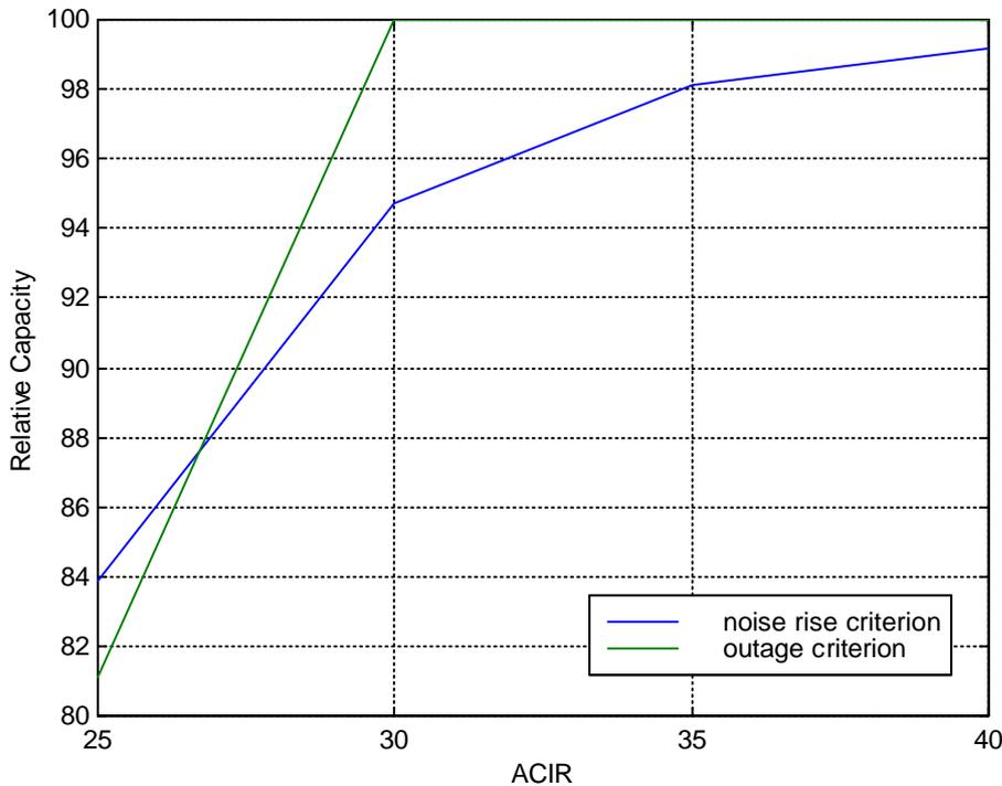
Figure 3. ACIR and capacity loss for UL speech service in the intermediate case applying the “satisfied user criterion”
