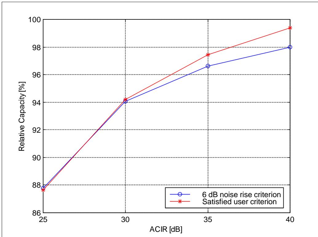
Figure 2. ACIR and capacity loss for UL 144 kbps data: worst case.
