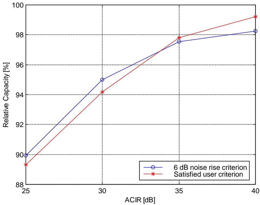
Figure 1. ACIR and capacity loss for UL 144 kbps data: intermediate case.
