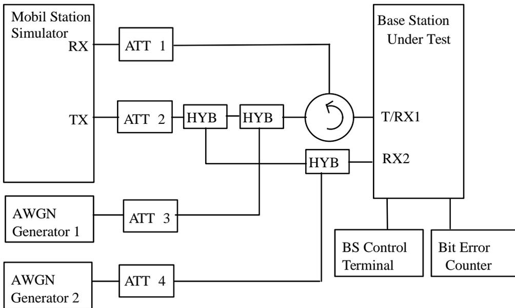
Fig. 6.1.2.7.2 Measuring system Setup for Base Station RSQI
