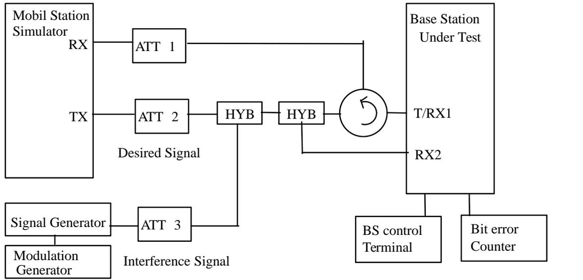
Figure 6.1.2.4.2 Measuring system Setup for Adjacent channel selectivity
