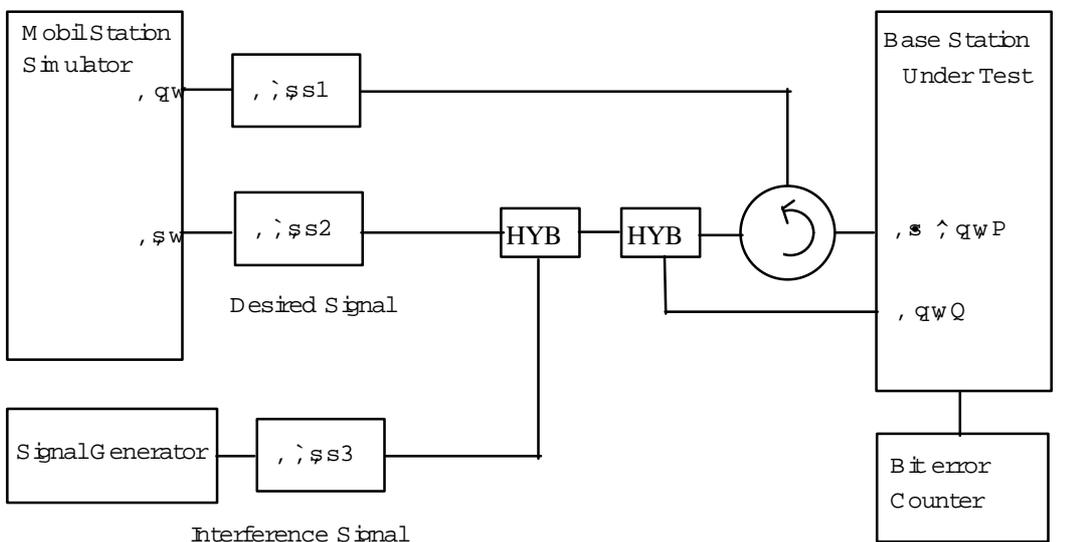
Figure 6.1.2.6.2 Measuring system Setup for Spurious Response
