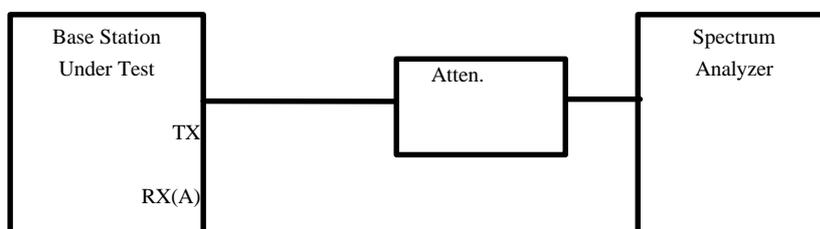
Figure 6.1.1.7-1 Functional Setup for Transmission on/off Ratio Test.
