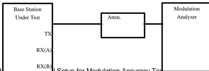
Figure 6.1.1.6-1 Setup for Modulation Accuracy Test.
