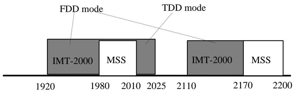
Fig. 2.1-2 Frequency band of ARIB-WCDMA System
