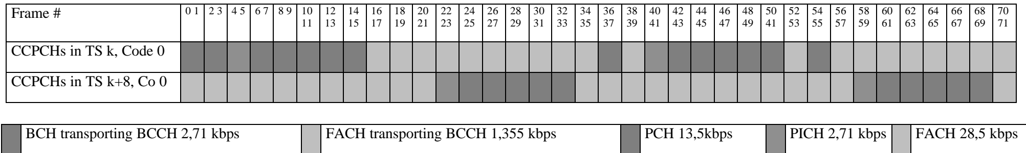
Figure B.3: Example for a multiframe structure for CCPCHs that is repeated every 72th frame
