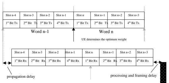
Node B receives the 4 Bits, Construct the Tx AA Word And Apply the same Tx AA Coeff. for the following 4 slots
