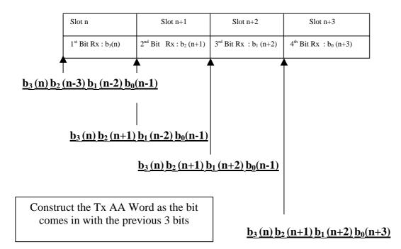
It is clearly seen from the progressive refinement at the UE that if the channel changes from one slot to another the UE can determine the new optimum coefficients for the current slot, thereby refining the Tx AA word sent.
