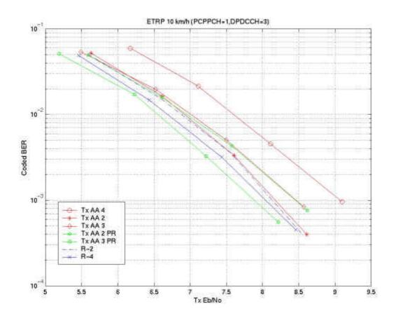
From the above results it is clearly seen that the progressive refine modes (PR) at the UE (MS) and Node B (BS) ameliorate quite significantly the current Modes as defined in the 3GPP Specifications both at low and high speeds. More importantly, they outperform the refined modes as proposed by Nokia.
