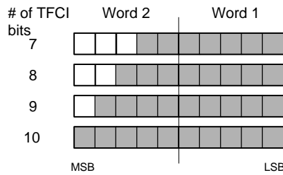
Figure Error! Style not defined.-Error! Bookmark not defined.. Mapping of TFCI bits to two words
