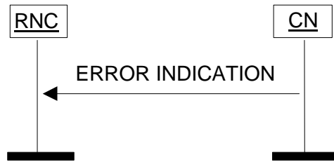
Figure 30 30 26 . Error Indication, CN originated.
