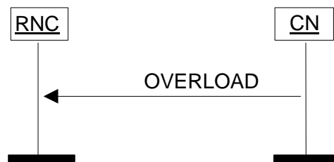
Figure 26 26 15 . Overload at the CN.
