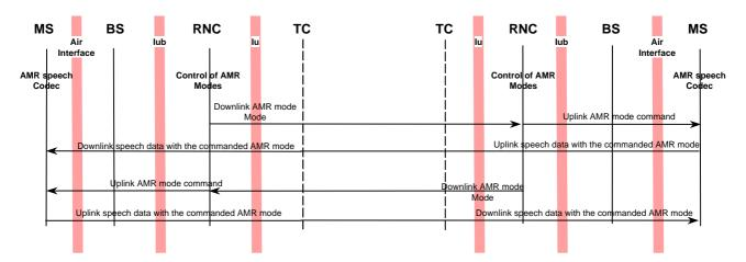
In this case, the local transcoder is not the final destination of the downlink codec mode command. The command must be transmitted (by some means) to the remote RNC to request the remote MS to use the best codec mode for the two involved systems. Note that in some cases, the remote network may be a GSM network also supporting in-band TFO or TrFO.
