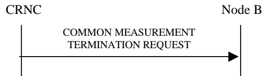
Measurement Termination Procedure initiated by RNC
