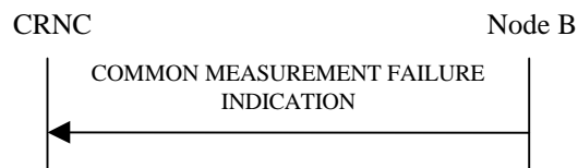
Measurement Failure Indication Procedure
