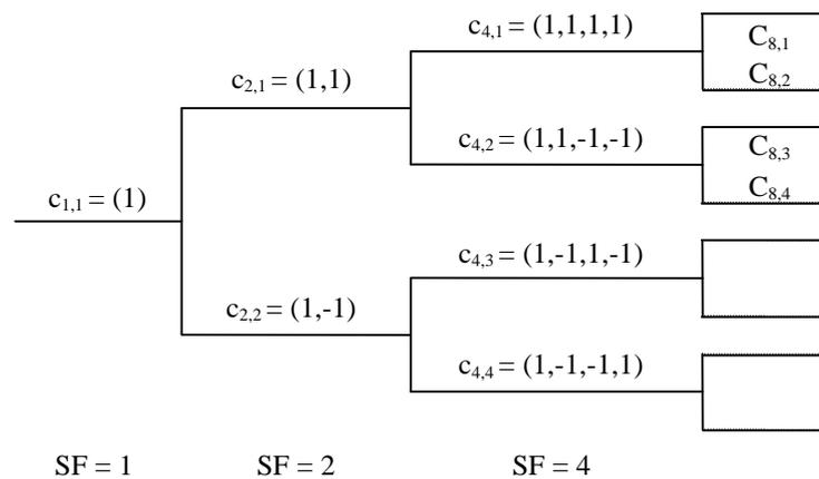
Fig. 1 Code-tree for generation of Orthogonal Variable Spreading Factor (OVSF) codes
