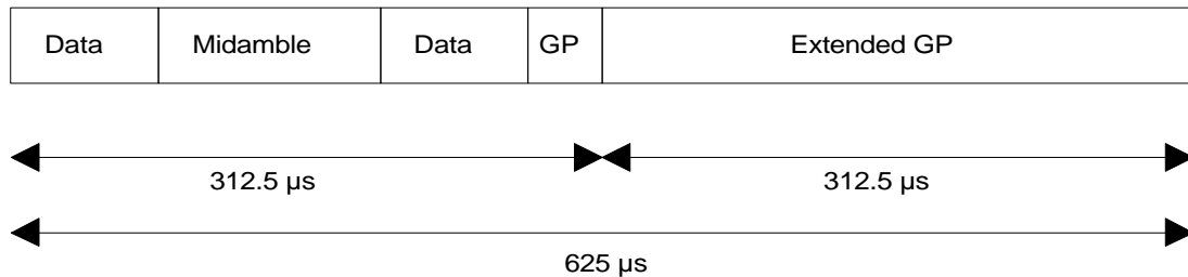
Figure 353 Access burst 1, GP denotes the guard period
