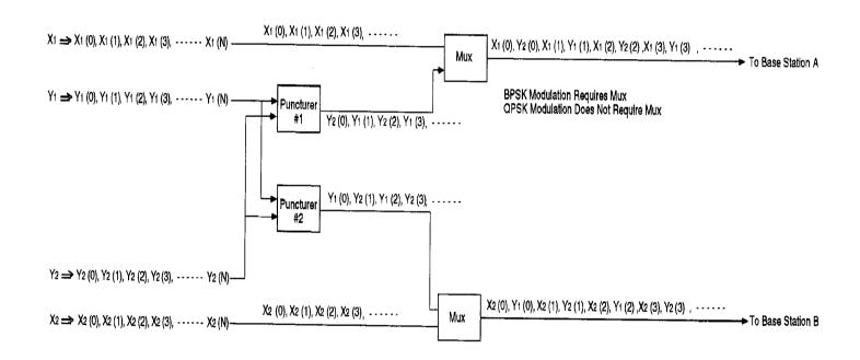
Puncturer #1 with Puncturing Pattern  $\begin{bmatrix} 0 & 1 \\ 1 & 0 \end{bmatrix}$ Puncturer #2 with Puncturing Pattern  $\begin{bmatrix} 1 & 0 \\ 0 & 1 \end{bmatrix}$
