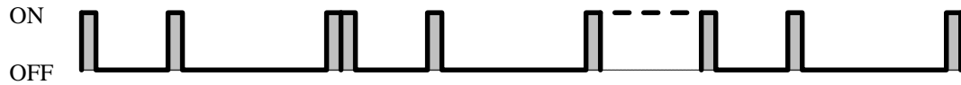
(iv) The whole DPDCH is power-off (no voice and no control information).
