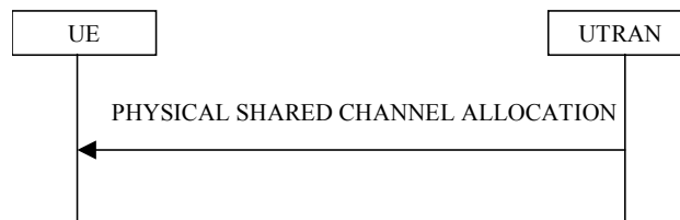
Figure 4-22: Physical Shared Channel Allocation procedure
