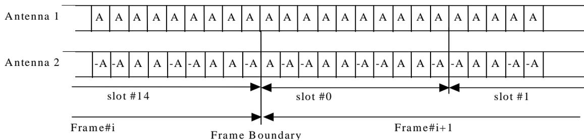
**Figure 14: Modulation pattern for Common Pilot Channel (with  $A = 1+j$ )**
