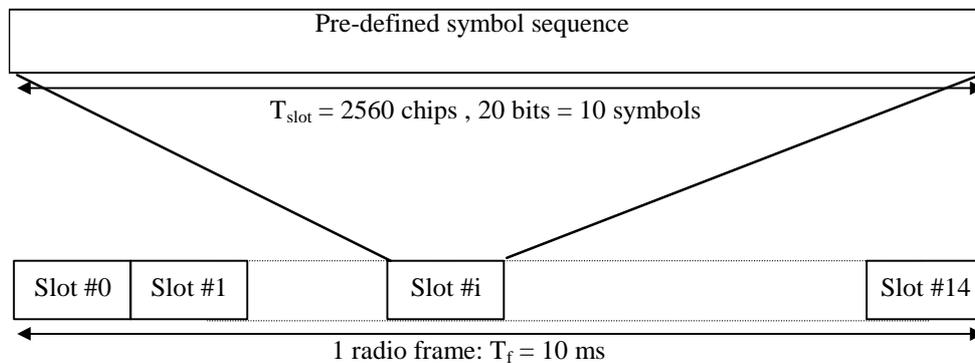
**Figure 13: Frame structure for Common Pilot Channel**
