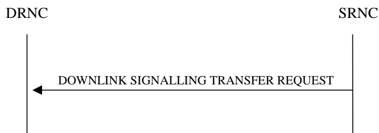
Figure 2: Downlink Signalling Transfer procedure, Successful Operation
