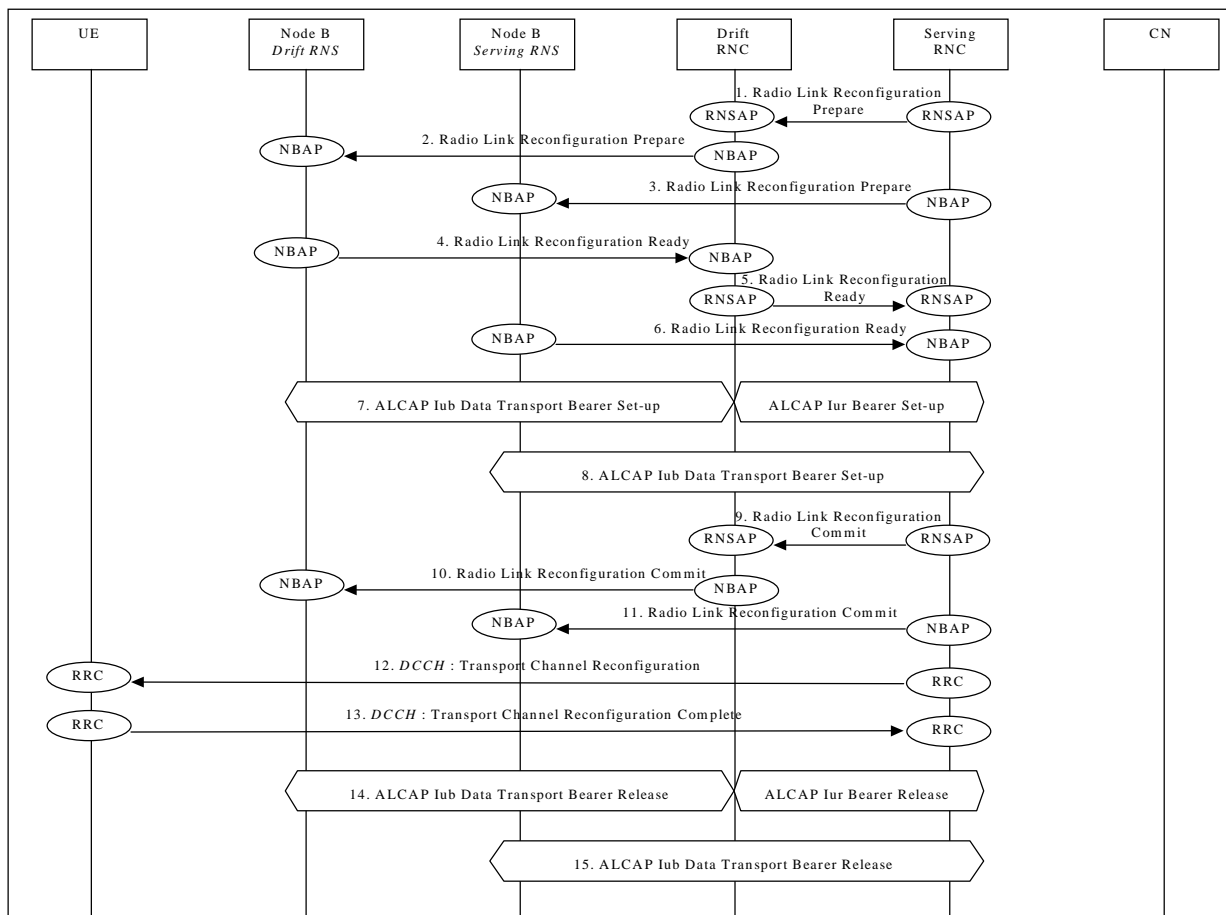
Figure 41: Synchronised Transport Channel Reconfiguration
