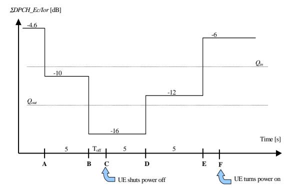
Figure 6.1. Conditions for out-of-synch handling in the UE. The indicated thresholds  $Q_{\text{out}}$  and  $Q_{\text{in}}$  are only informative.
