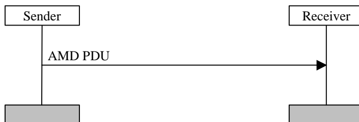
Figure 11.3: Acknowledged mode data transfer procedure
