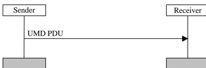
Figure 11.2: Unacknowledged mode data transfer procedure
