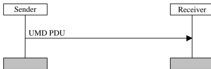
Figure 11.2: Unacknowledged mode data transfer procedure
