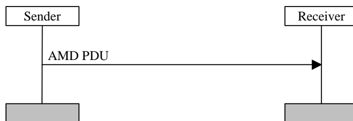
Figure 11.3: Acknowledged mode data transfer procedure
