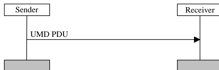
Figure 11-2: Unacknowledged mode data transfer procedure
