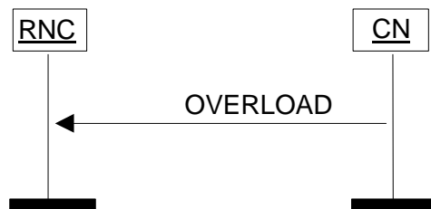
Figure 48 26 15 . Overload at the CN.
