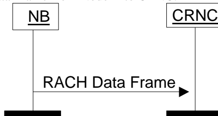
Figure 1. RACH Data Transfer Procedure.
