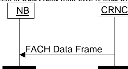
Figure 2. FACH Data Transfer Procedure.
