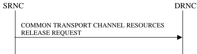
Figure 9-17: Common Transport Channel Release
