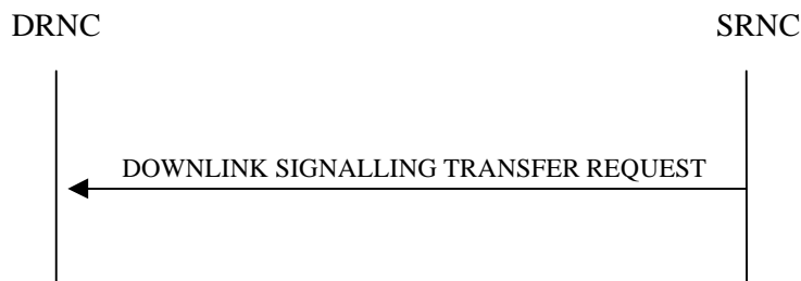
Figure 9-9: An example RNSAP message flow at I ur interface for Downlink Signalling Transfer
