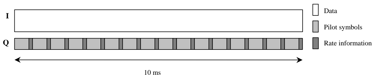
Figure 4: The message part of the random-access burst.
