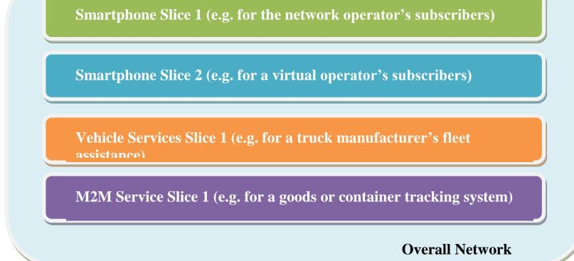
Slicing enables the operator to deploy multiple, more or less independent end-to-end networks potentially with the same infrastructure.
