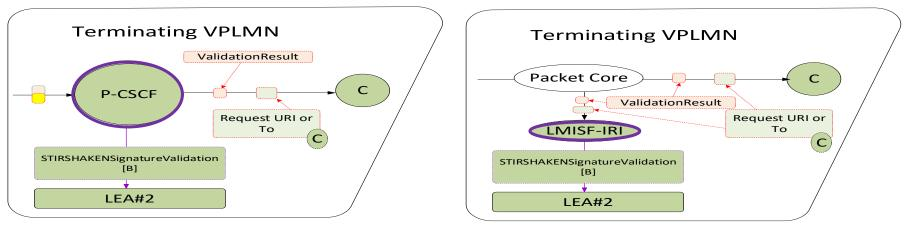
The IRI-POI present in the LMISF-IRI or P-CSCF (VPLMN) shall generate an xIRI containing a STIRSHAKENSignatureValidation record when the following conditions are met:
