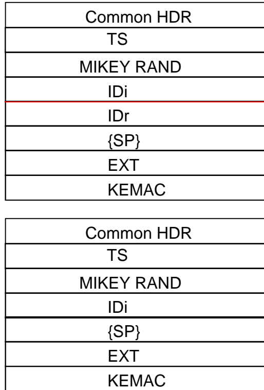
Figure 6.5: The logical structure of the MIKEY message used to deliver MSK. For use of brackets, cf. section 1.3 of RFC 3830 [9] (MIKEY)
