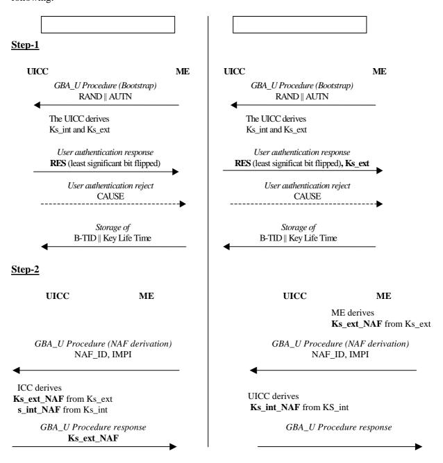
In case of Ks\_ext stored on the UICC, another alternative to derive Ks\_xx\_NAF keys was proposed at SA3#34. This solution is described in section 3.6 of the present document. Besides an analysis of the key derivation alternatives is provided in another SA3#35 contribution [2].
