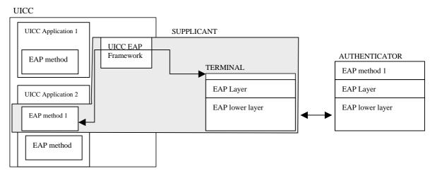
Figure 1: EAP architecture when supplicant is split between a UICC and a terminal.
