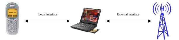
The mobile phone (the "card holding device") on the left holds the UICC or SIM (the "card") and the laptop holds the WLAN card.
