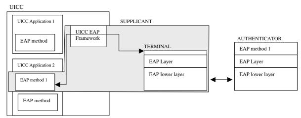
Figure 1: EAP architecture when supplicant is split between a UICC and a terminal.
