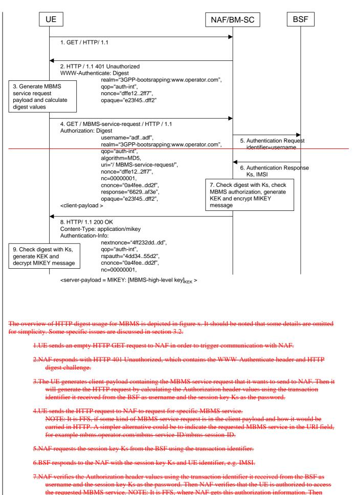
NAF generates the KEK and integrity key using Ks as key material and using functionality specified in MIKEY. Then NAF generates the MIKEY message including the high level MBMS key and protects it with the KEK and the integrity key.
