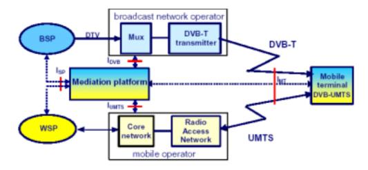
A "Mediation Platform" function will exist between the two paths to allow sharing and re-directing of data. Content can be re-purposed and transferred between platforms (eg. DVB content delivered via UMTS), and opportunities for exciting new application exist."
