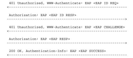
Figure 1. HTTP EAP Authentication message flow
