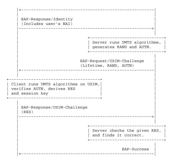
When EAP AKA is run in the GSM compatible mode, the message flow is otherwise identical to the message flow below except that the AUTN parameter is not included in EAP-Request/USIM-Challenge packet.
