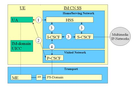
The protocol used between the UE and the P-CSCF is SIP, Session Initiation Protocol. A working assumption in SA3 has been that AKA defined in R'99 shall be reused. However, currently within IETF SIP AKA has not been defined. In SA3 #14 Nokia presented a proposal [S3-000456] on how AKA could fit into the SIP protocol by extending the protocol. That is also the current working assumption.
