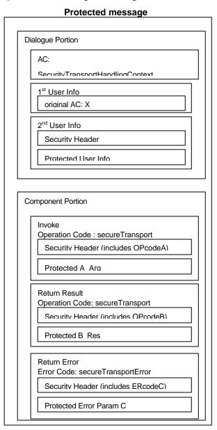
As it can be seen, it is proposed to protect each component of the message separately with the possibility to specify a different Protection Mode level at the Security Header of the different message components.
