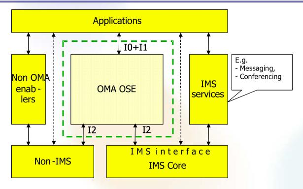
3GPP/3GPP2 have also standardized sevice capabilities to offer IMS services that work on top of the IMS core, and thus at the same architectural level as OMA enablers. These IMS services may be good candidates for OMA enablers, in order to provide capabilities that are currently not in the set of existing or ongoing OMA enablers.
