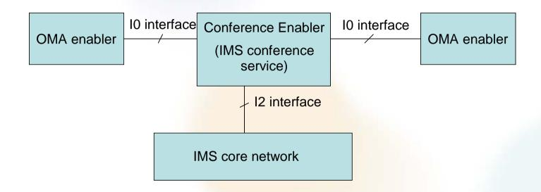
If an IMS service is found to be a good candidate for an enabler that does not exist yet, it can be integrated in the OSE by identifying I0 interfaces for it (I2 interfaces, to IMS Core, would already be specified)
