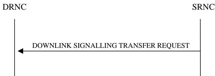
Figure 29-9: An example RNSAP message flow at I ur interface for Downlink Signalling Transfer
