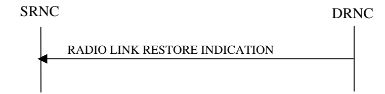
Figure 12: RL Restoration procedure
