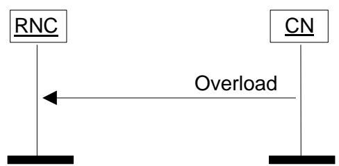
Figure 466. Overload at the CN.
