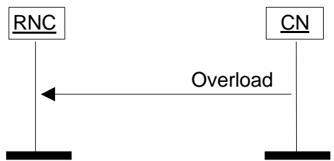
Figure 6. Overload at the CN.
