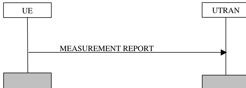
Figure 2) Measurement Report procedure
