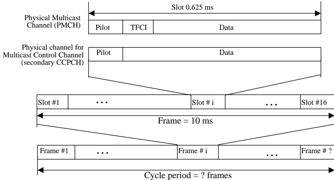
[Figure 3 Physical Channel Structure for multicast]
