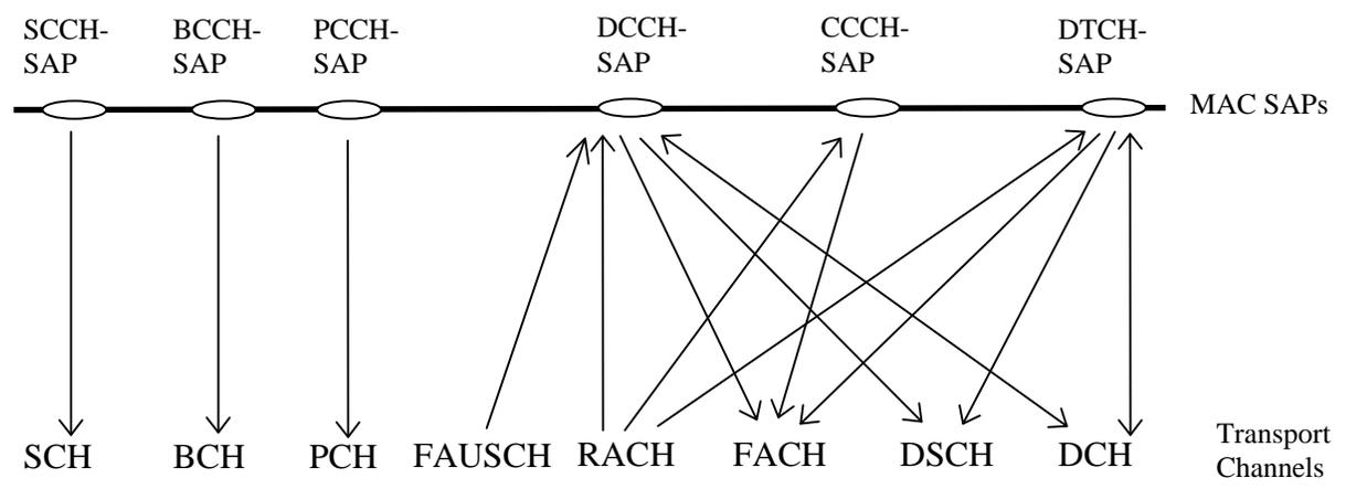
[Figure 4 Logical Channels to Transport Channels, UTRAN side]
